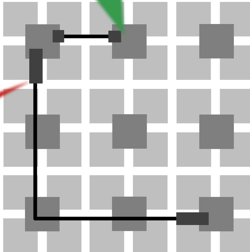
✗ Long wire: traversing the whole die requires large input buffers for full link utilization
