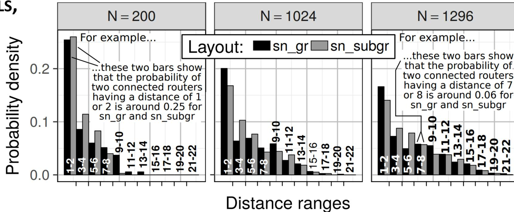
**Figure 6.** (§ 3.3) Distribution of link distances in SNs. A bar associated with a distance range  $X$  illustrates the probability that, for a given layout, two routers are connected with a link that has the distance falling within  $X$ . Bars of different colors are placed pairwise so that it is easier to compare the subgroup and group layouts.
